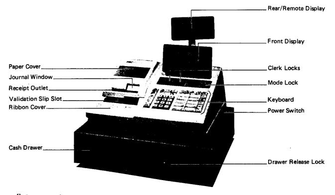
[] Power Switch ... The power switch is provided at the righthand side of the cabinet. The AC power is turned on when the switch is pushed to ON, and turned off when the switch is pushed to OFF.
